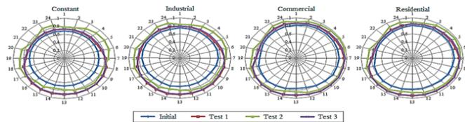
**Fig. 6.** The variation of voltage stability on 69-bus distribution system with consideration the weather conditions
