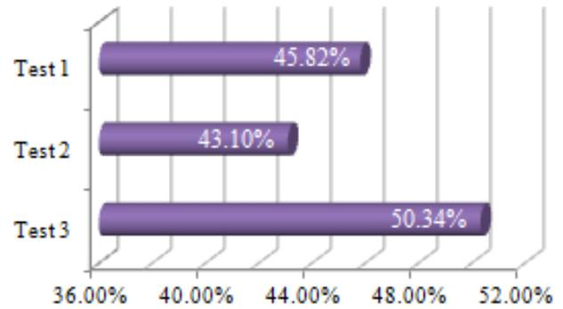
Fig. 9. Improved percentage of actual network loss after placement of devices
