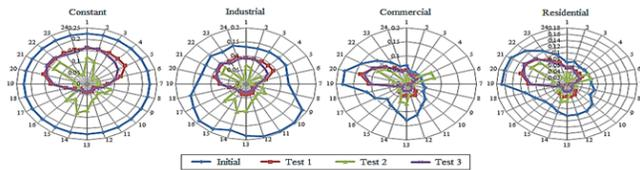
**Fig. 5.** The variation of active loss on 69-bus distribution system with consideration the weather conditions
