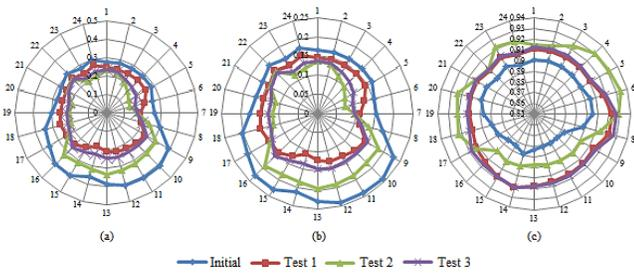
**Fig. 11.** The variation of technical indices of 101-bus system with consideration the weather conditions (a) Active loss (b) Reactive loss (c) Voltage stability
