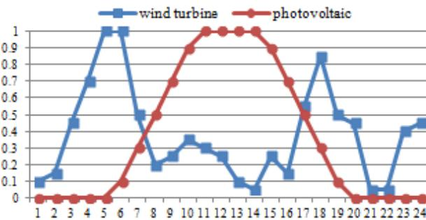
**Fig. 3.** The variation of production of wind turbine and photovoltaic (Pu)
