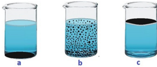
Fig. 1. Schematic of (a) underfloor heating mode; (b) nanofluid mode (c) floating mode of solar steam generation
