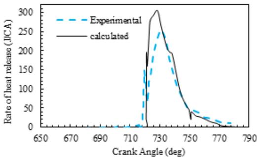
**Fig. 3.** Comparison of the experimental [14] and calculated RHR for the ISM 370 engine (maximum error by 10%)
