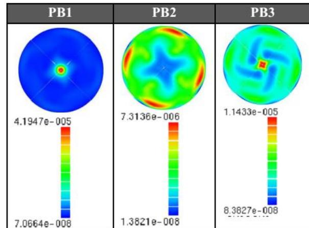
**Fig. 15.** Unburned DME mass fraction in combustion chamber almost when the exhaust valve is opening under 1400 rpm engine speed
