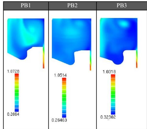
**Fig. 11.** Equivalence ratio distribution almost when the exhaust valve is opening for different piston bowls
