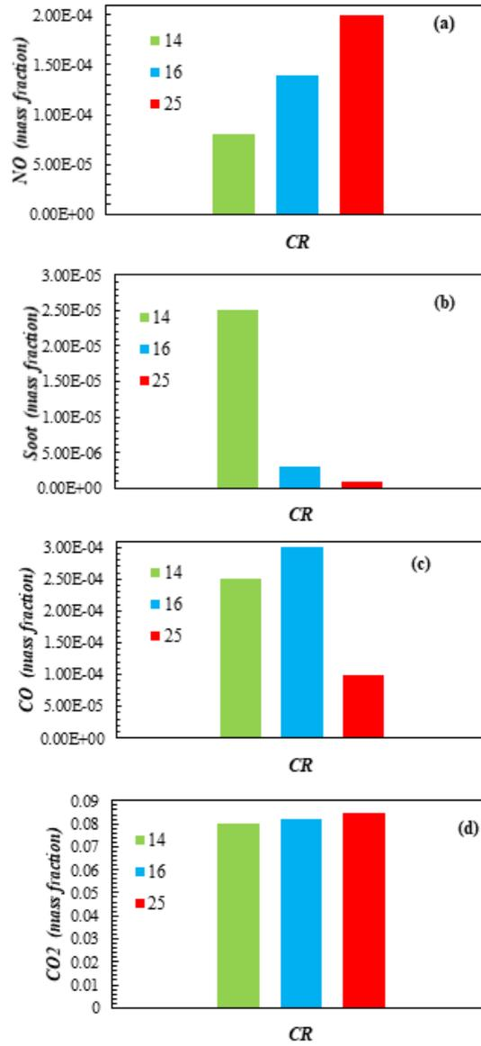
**Fig. 19.** Influences of changing the CR on emission characteristics under 1400 rpm engine speed (a): NO mass fraction (b): soot mass fraction (c): CO mass fraction (d): CO2 mass fraction
