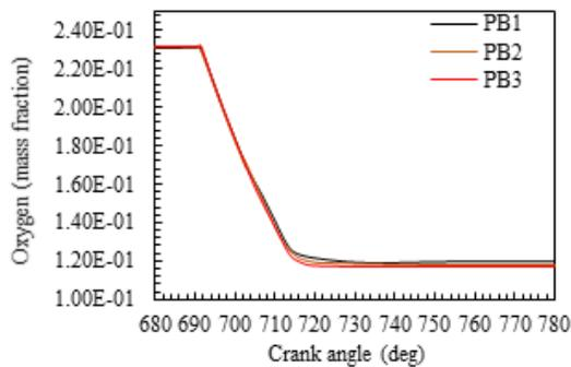
**Fig. 14.** The oxygen mass fraction under 1400 rpm engine speed
