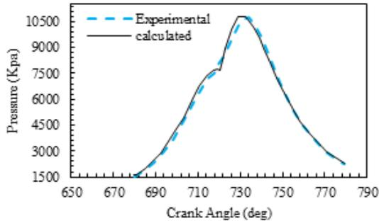
**Fig. 2.** Comparison of mean pressure between experimental [14] and predicted data for the ISM 370 engine (maximum error by 5%)
