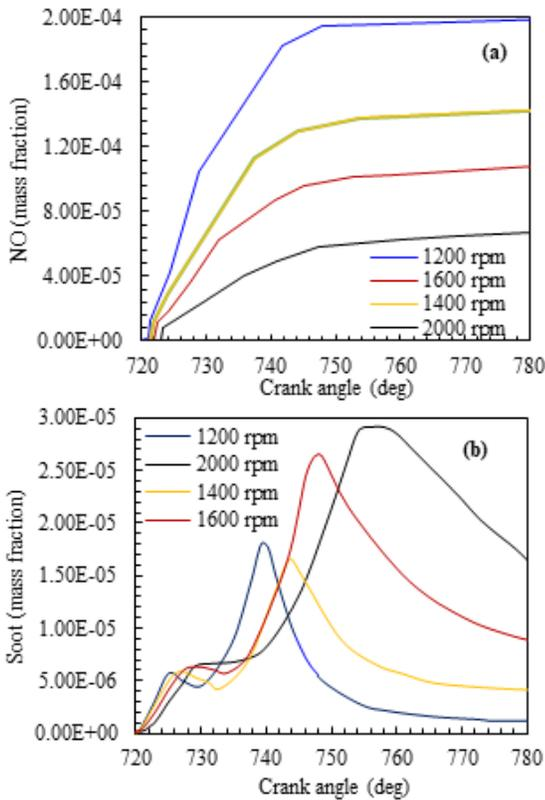
**Fig. 7.** The engine speed effects on soot and NO emissions (PB2) (a): mass fraction of NO (b): mass fraction of soot
