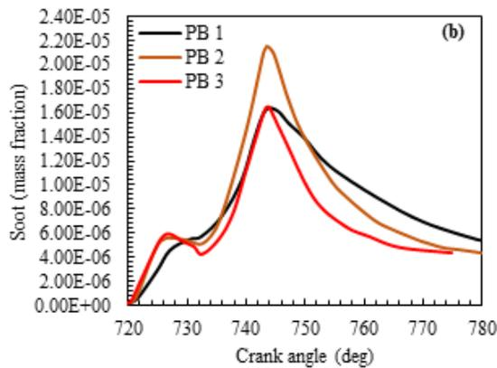
**Fig. 10.** The piston bowl geometry effects on NO and soot mass fraction (a): NO mass fraction (b): soot mass fraction
