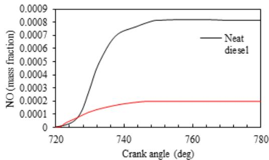
**Fig. 21.** NO emissions for DME and diesel fuel
