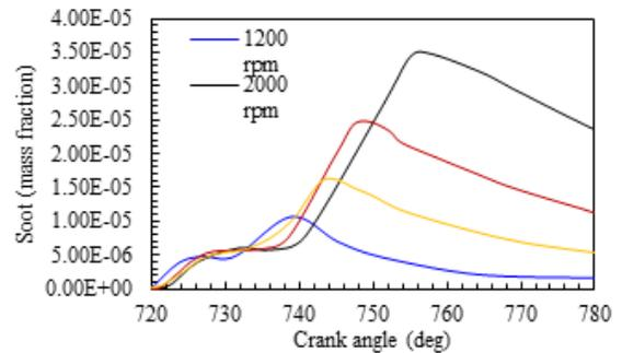
**Fig. 6.** The engine speed effects on soot emissions (PB1)
