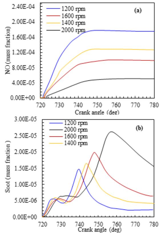
**Fig. 8.** The engine speed effects on soot and NO emissions (PB3) (a): mass fraction of NO (b): mass fraction of soot
