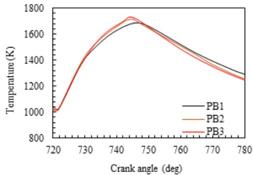
**Fig. 13.** The mean temperature in cylinder under 1400 rpm engine speed
