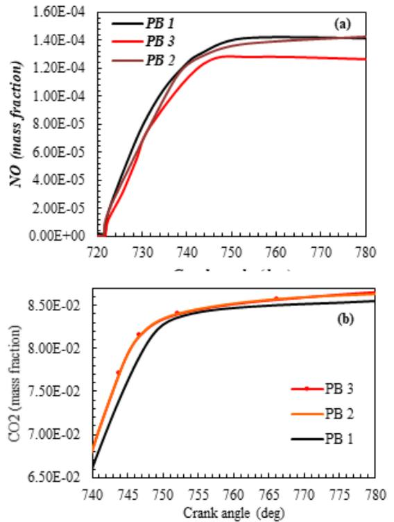
**Fig. 12.** Effect of changing the piston bowl geometry on the (a): CO and (b): CO2
