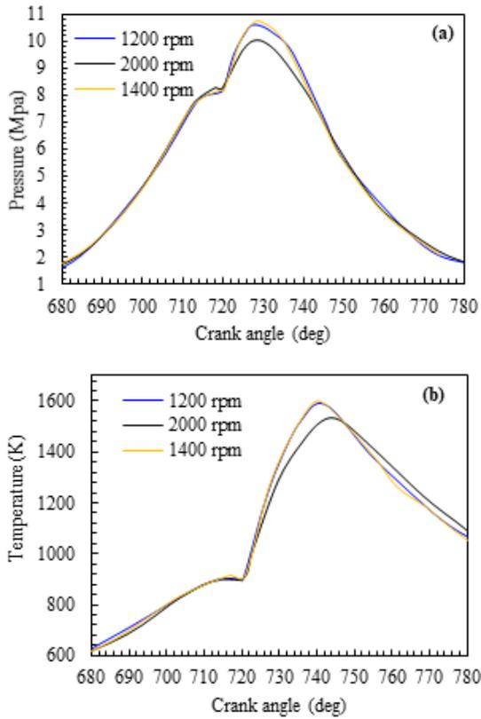
**Fig. 9.** The engine speed effects on in-cylinder mean pressure and temperature (a): mean pressure (b): mean temperature
