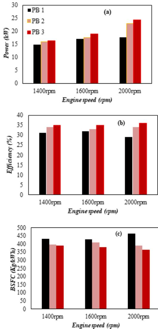
**Fig. 16.** Comparison of power, thermal efficiency and BSFC under engine speeds of (a):1400 rpm, (b): 1600rpm, and (c): 2000 rpm
