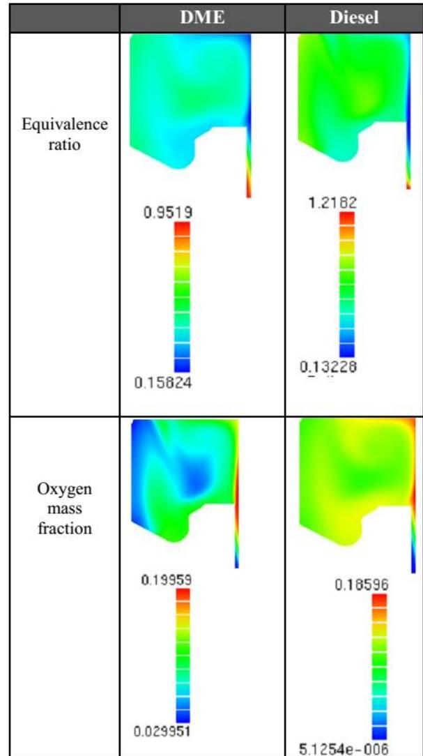
Fig. 24. Equivalence ratio (ER) and oxygen mass fraction distributions almost when exhaust valve is opening for diesel and DME fuel
