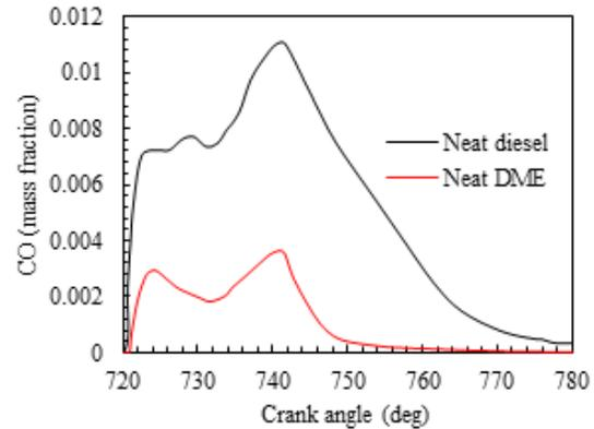
**Fig. 22.** CO<sub>2</sub> and CO emissions for DME and diesel fuel (a): CO<sub>2</sub> (b): CO
