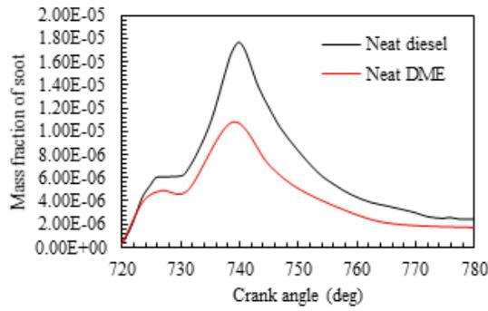
Fig. 23. Soot emissions for DME and diesel fuel
