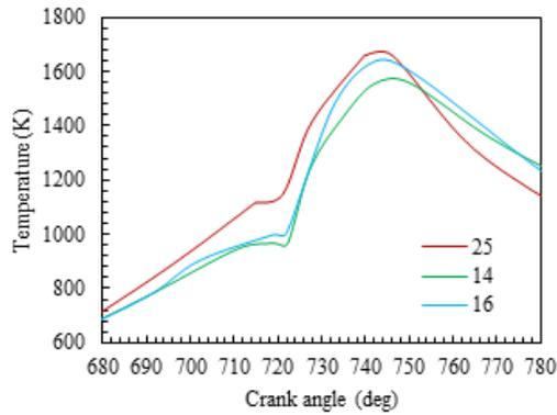
**Fig. 20.** Cylinder temperature curves under different compression ratios.
