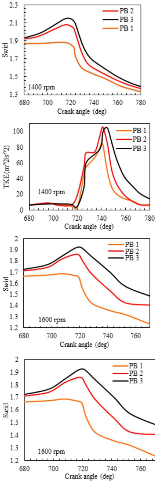
**Fig. 17.** Distribution of swirl and TKE versus crank angle for three piston bowl geometries under 1400 and 1600 rpm engine speeds
