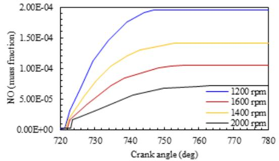
**Fig. 5.** The engine speed effects on NO emissions (PB1)
