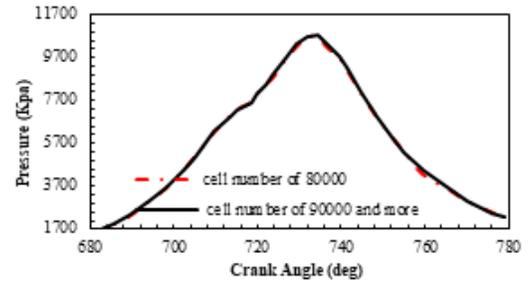
**Fig. 1.** Comparison of the cylinder pressure curves after cell number of 80000.
