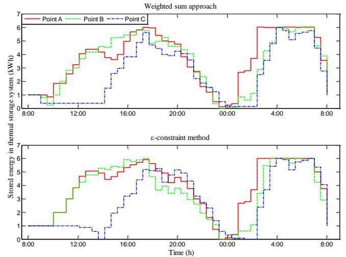
Fig. 9. Amount of stored heat in the thermal storage system
