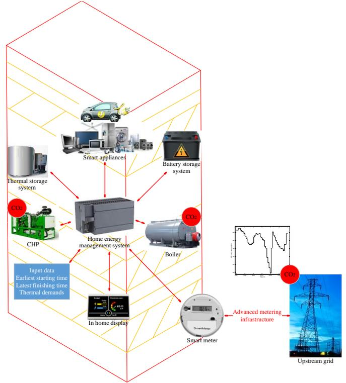
Fig. 1. Overall architecture of the smart apartment building model
