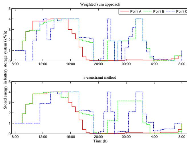
Fig. 7. Amount of stored energy in the battery storage system
