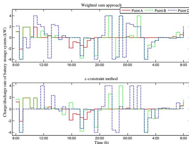
Fig. 8. Charge and discharge rates of the battery storage system
