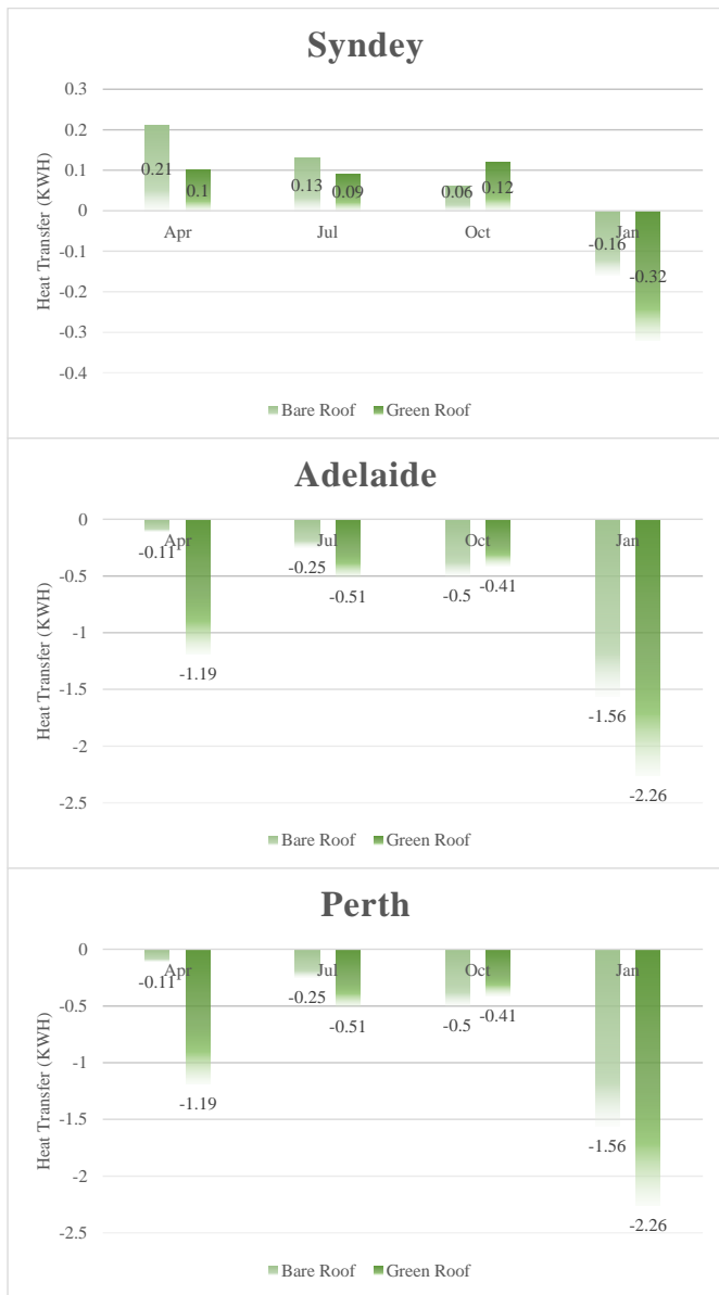
Fig. 13. Heat transfer of bare and green roof for each city in different months.
