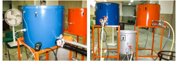
Fig. 6. OET Open expansion tanks pilot in the energy auditing lab. (1) Optimized model by the coil. (2) Conventional model. (3) Optimized Twin container
