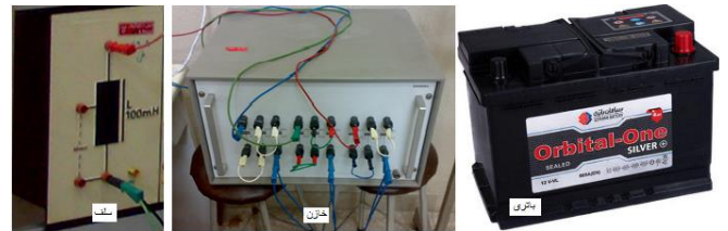
Fig. 29. Battery, capacitor and filter inductance in the charger.
